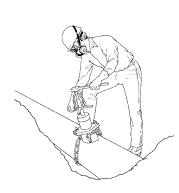
Pressure or "wet" tapping for service connections is performed in the trench while the pipe is under pressure. The equipment (manual driven) is affixed to the pipe by means of a chain yoke. A combination boring-and-inserting bar drills and taps the pipe wall and inserts a corporation stop or pipe plug. The pressure chamber, which protects against water leakage, also catches the asbestos-cement chips, so this is essentially a dust-free operation.
