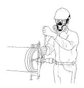
Manual field lathes are designed to end-trim and re-machine rough pipe barrels to factory-machined end profiles. The lathe consists of an adjustable, self-aligning arbor inserted into the pipe bore (which acts as a mandrel upon which the turning handle operates), a screw-fed turning frame, carbide machining blades, and manual (hand or ratchet) turning handles.
